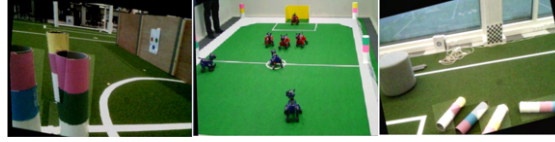
Figure 3.7: Some examples of images from the dataset after image augmentation. The leftmost and rightmost images contain the landmarks on the same Nao robot football field on which the final dataset is recorded with a rotation, bounding box brightness, and a minimal bounding box rotation. The centre image contains a picture of a smaller Aibo football field with bounding box brightness.
