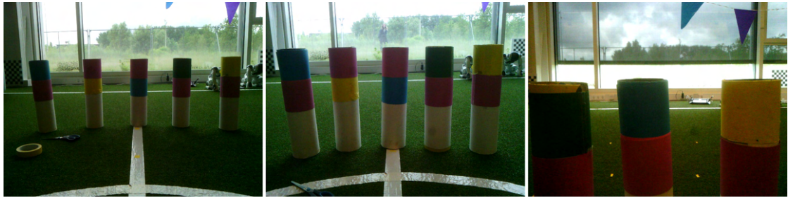
Figure 3.5: Field landmarks placed at a certain distance at different angles from the robot. From left to right: 150cm at \pm 20^\circ , \pm 10^\circ and 0^\circ , 100cm at \pm 20^\circ , \pm 10^\circ and 0^\circ , 50cm at \pm 20^\circ and 0^\circ .
