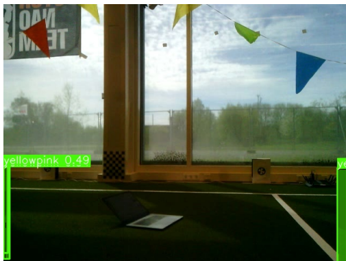
(c) Example of false positives detected with the small model. Yellow-pink was detected three times, two times in the left pole, with confidences 48.6% (marked as true positive) and 34.0% (marked as false positive), one time on the right side, with confidence 27.5% (marked as false positive). The wrongly classified green-pink landmark is marked as a false negative.
