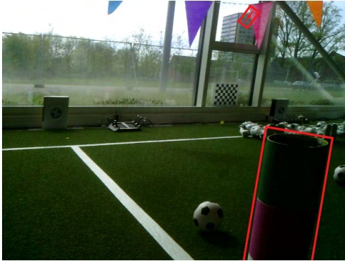
(a) Example of a false positive detection in the pink flag and the building, as well as a false negative detection of the green landmark
