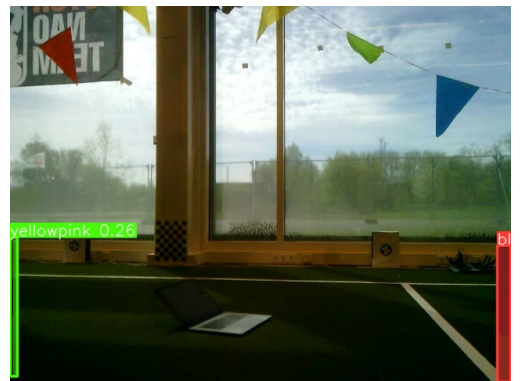
(d) Example of false positives detected with the medium model. Yellow-pink was correctly detected one time with a confidence of 25.9%. The green-pink landmark is classified as a blue-pink landmark with confidence 49.5%, marked as a false positive. The wrongly classified green-pink landmark is marked as a false negative.
