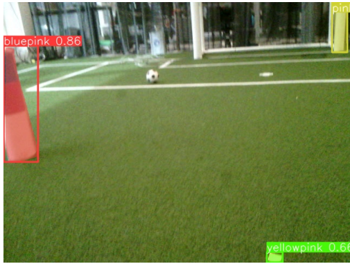
(a) Example of false positives detected with the small model. Blue-pink detection: true positive, confidence: 85.7%. Yellow-pink detection in the tape on the field: false positive, confidence: 66.3%. Pink-yellow detection in the goal post: false positive, confidence: 49.1%.
