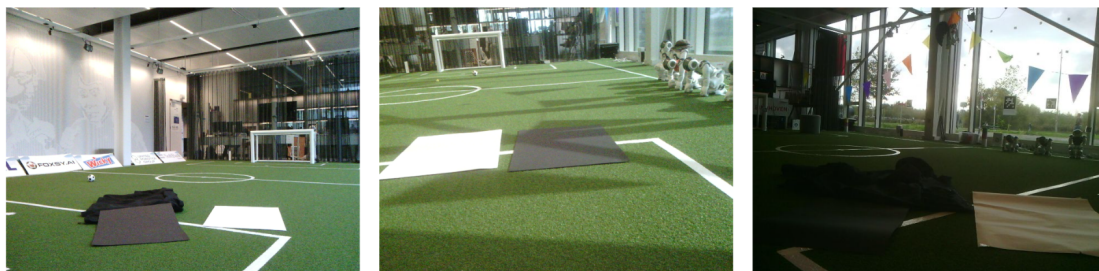
Figure 8: Three scenarios for color calibration under varying lighting conditions. From left to right: (1) Homogeneous lighting with consistent color values, (2) High variance in color values due to uneven lighting, and (3) A challenging case where colors (green, black, and white) have similar pixel values, making detection difficult.
