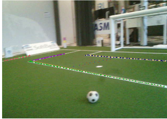
Figure 11: An example of lines and inlier line spots found by the line detector. A merge test is also performed between the outer lines of the goal area and the penalty area.
