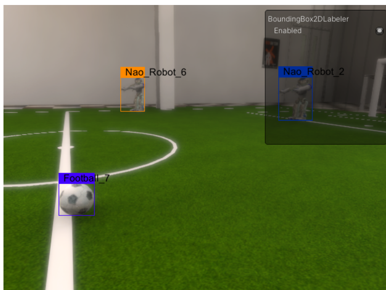
Figure 1.1: A screenshot of the Unity camera window. The bounding boxes and classes are determined and visualized using the Perception package.
